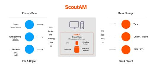
ScoutAM is the only mass storage platform built on a converged metadata architecture, meaning that metadata is stored within the application stack. Other products utilize a diverged model wherein metadata is handed off to a separate third-party database tool like Cassandra, or DB2 for storage and processing. Many of the legacy mass storage systems refer to their metadata collection as "the database", reflecting the fact that the metadata is managed by a separate tool.
