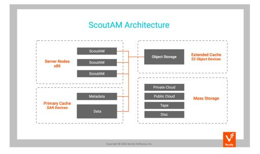
The ScoutAM platform is deployed on standard hardware components in five functional categories.
