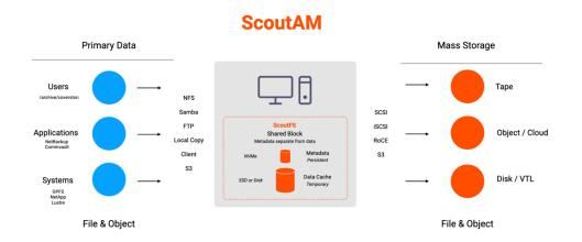
ScoutAM is the only mass storage platform built on a converged metadata architecture, meaning that metadata is stored within the application stack. Other products utilize a diverged model wherein metadata is handed off to a separate third-party database tool like Cassandra, or DB2 for storage and processing. Many of the legacy mass storage systems refer to their metadata collection as "the database", reflecting the fact that the metadata is managed by a separate tool.
